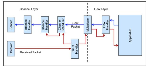
Fig. 6. Internal packet and data flow diagram
