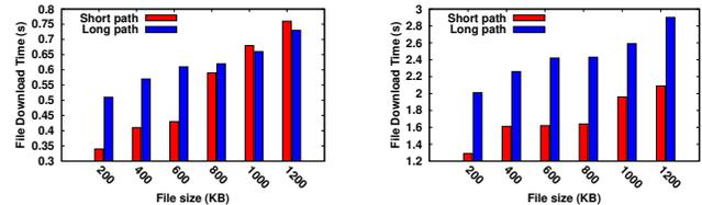
Fig. 2. File download time when short path is the primary path vs when long path is the primary path
