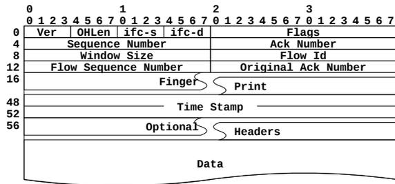
Fig. 5. Viscous packet header structure
