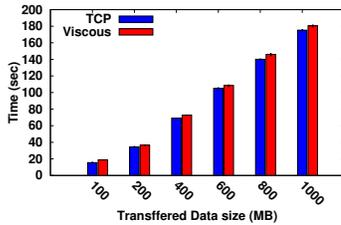
Fig. 13. Performance of Viscous and TCP for long flows over a single path
