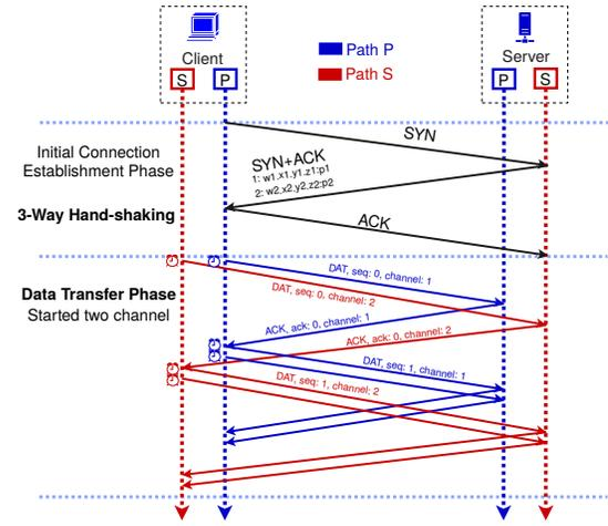
Fig. 4. Three-way handshaking between client and server and data transfer between them. Handshaking can go between any two pairs of interfaces. Here P is the primary path and S is one of the secondary or alternative paths.
